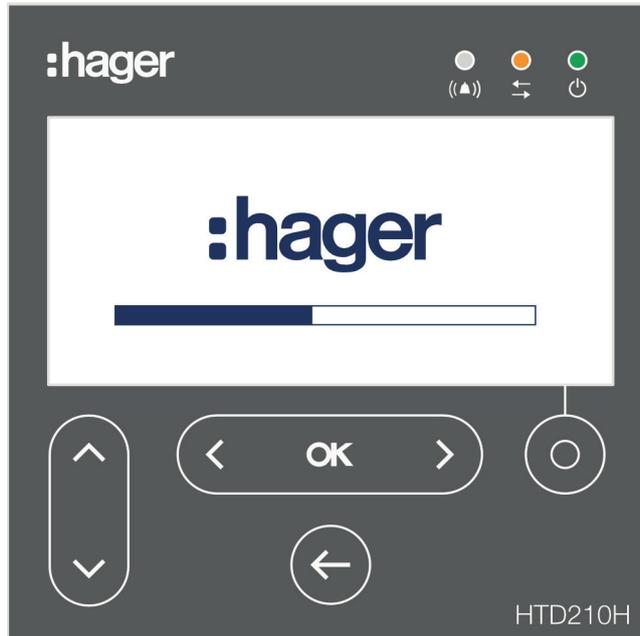
While the Start up screen is displayed, the Panel display is fetching its configuration settings stored in the Energy MCCB. If the stored data is corrupted or empty (e.g. on first power up), default values will be set.
