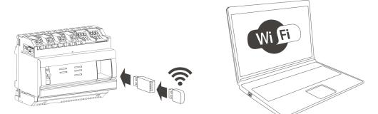
The HTG460H WLAN dongle is a USB to Wi-Fi interface, especially suitable for the connection without wire with the HTG410H. It allows direct connection on the front panel. This is the easiest mean to connect a computer or a tablet.
