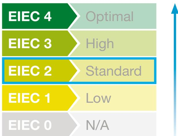
Since October 2015, the energy efficiency of electrical installations has to be evaluated according to the classification procedure laid down in IEC 60364-8. This yields an energy efficiency class for the entire electrical installation – EIEC 0 to 4.
