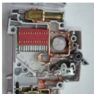
A counterfeit of a Hager circuit breaker without magnetic and thermal trip.
