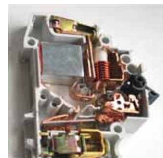
A copy of a Hager circuit breaker with a massive steel arc chamber.
